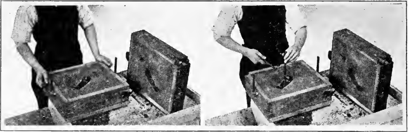
FIG. 508. COPE LIFTED OFF.
